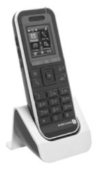
Put your phone on its support. Plug the USB cable into the 5V socket of the desk support. Plug the other end of the USB cable into the AC/DC adapter. Plug the adapor into the mains power supply.
