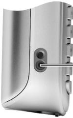
After removing the plastic cover, you can connect a headset to the left-hand side of your handset with the 2.5 mm jack connector.
