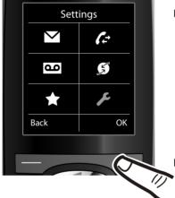
Use the right, left, down and up control key to navigate to the Settings submenu.
