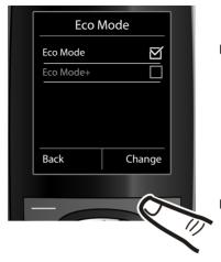
▶ Press down on the control key until the Eco Mode+ menu appears on the display.
