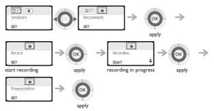
While recording a comment you can select other functions using the navigate-up-down key
